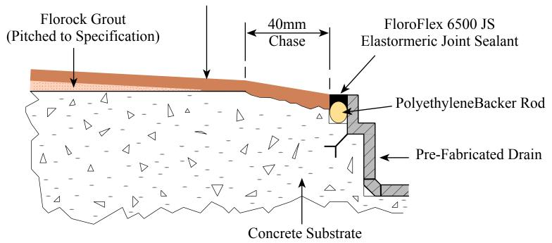
Note: Backing Rod positioned to provide an installed sealant depth that is equal to 50% of the joint width.
