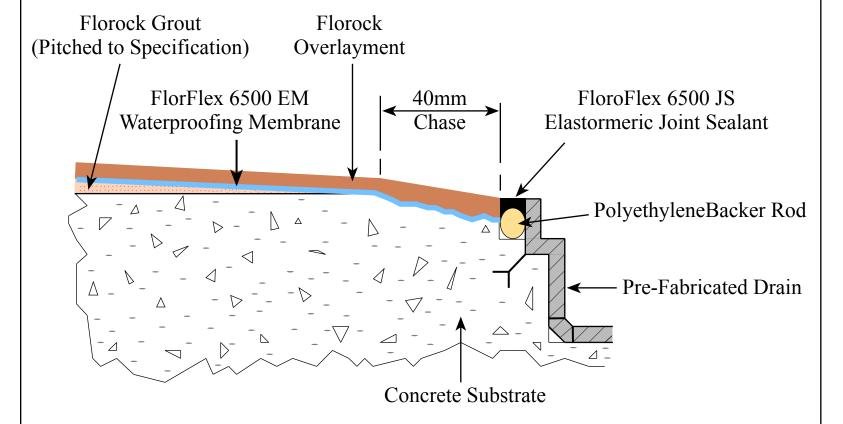
Note: Backing Rod positioned to provide an installed sealant depth that is equal to 50% of the joint width.
