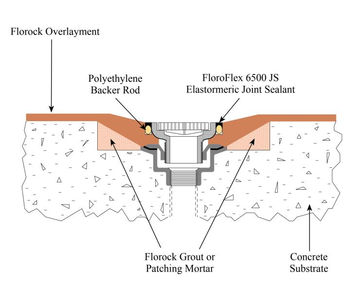
Note: Backing Rod positioned to provide an installed sealant depth that is equal to 50% of the joint width.
