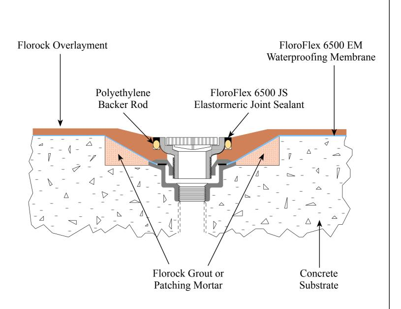
Note: Backing Rod positioned to provide an installed sealant depth that is equal to 50% of the joint width.
