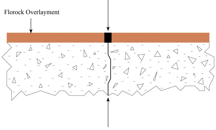
Control or Construction Joint with Potential Movement
